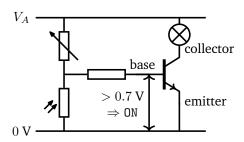
The variable resistor may be used to alter the light level at which the transistors switches on (higher R means lower V across LDR for a given light intensity).
